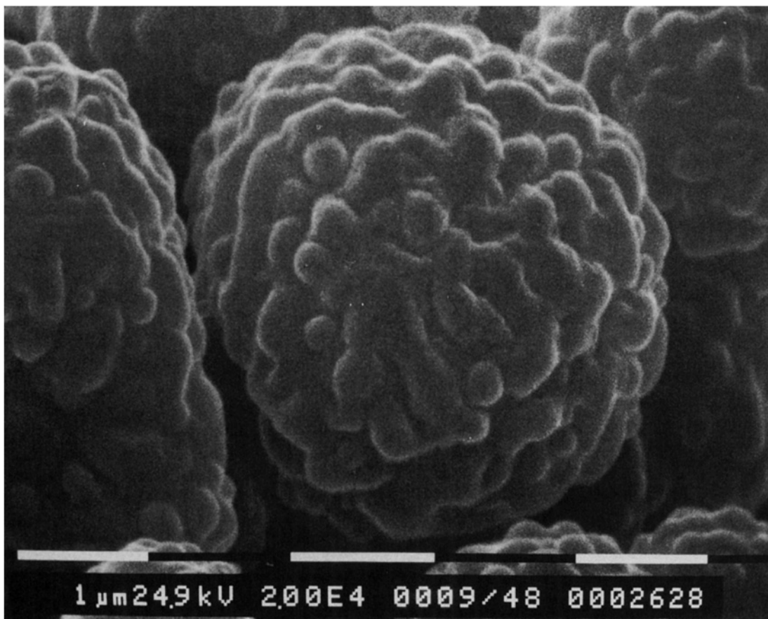
Figure 6 Primary particle of PVC from suspended emulsion polymerization (high magnification: white bar = 1 micron).
